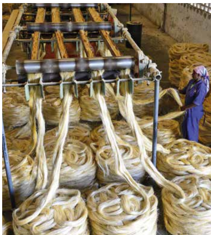
The spinning unit at Tancord (1998) Limited. The fibres are subsequently turned into carpets, doormats, cables, ropes, hawsers, nets sacks and yarn.
